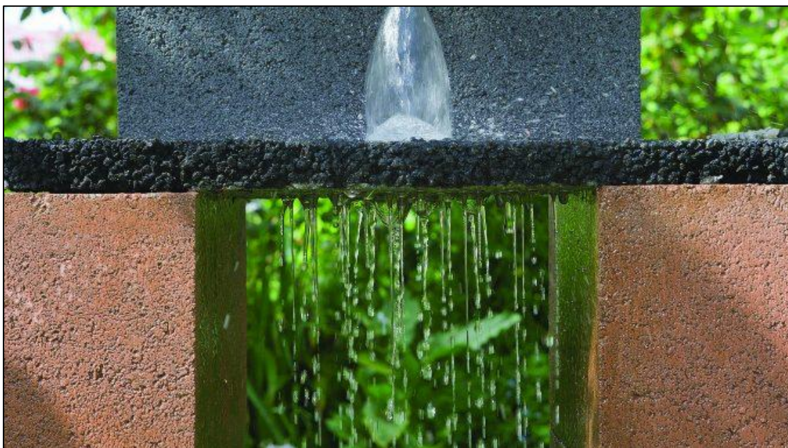
Figur 8. Infiltration genom permeabel asfalt (Magazine.ogind.com, 2018).
